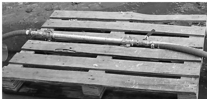
Figure 1. Side stream overflow pipe arrangement
